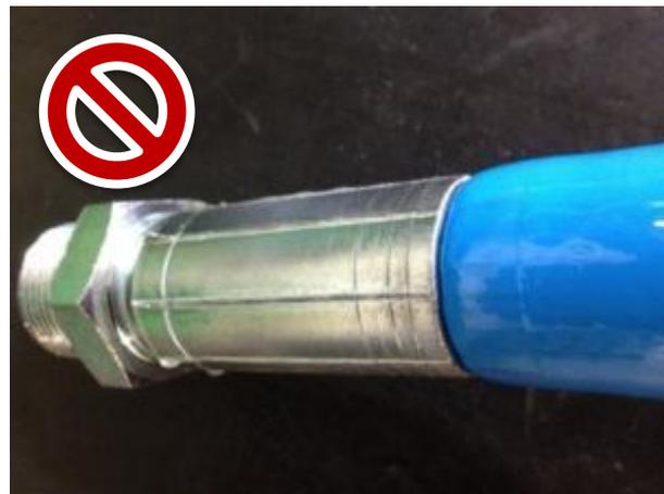
*Effects of under swaged and over swaged hose respectively. Follow the specified swage OD.*
