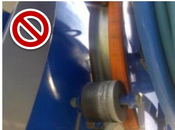
*A severely damaged hose due to a bad routing and setting of the guide on the truck.*
