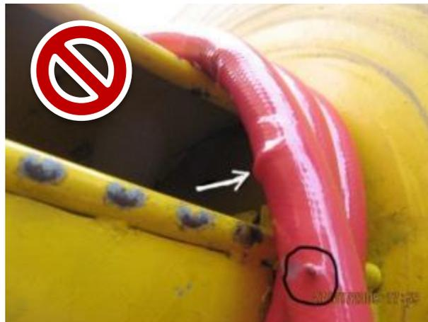
*Unsuitable hose drum could squash and damage the hose during application. The white arrow and the black circle underline the effect of this improper use.*
