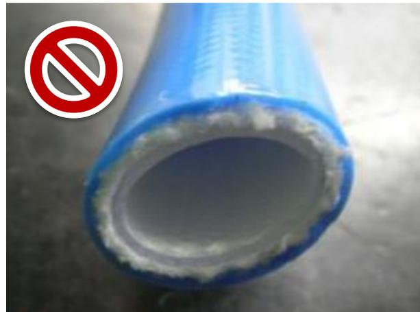
*Do not allow the hose to be run over by vehicles. Driving over a sewer hose may squash the hose and damage it irreparably. The second image shows effect on shape of a hose excessively squashed.*
