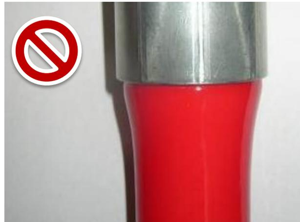
*The first image shows the normal appearance of a no-stretched hose. The second image shows the distortion of the hose due to an excessive stretching.*
