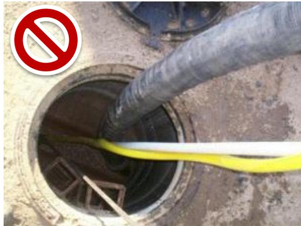
*A hose with a severe cover cut, probably produced by sharp edges inside the sewer.*
