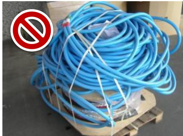
The first image represents some hoses well stored. These hoses are coiled onto a wooden bobbin or neat coil, protected from dust and environmental factors with protective packaging. The second image shows an improper storage. This hose could be severely damaged and also could be a danger for people that work close to the hose.
